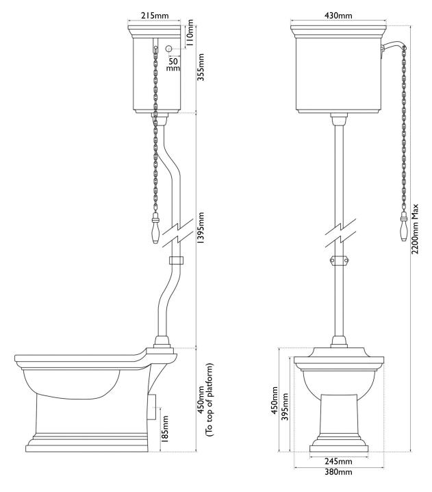
Chichester flush pipe = 1495mm (-100mm hidden in cistern & pan) Exposed length = 1395mm
